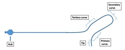
**Figure 1.** Basic construction of a catheter. Catheter consists of a hub at the rear end and a distal tubular shaft. The shaft can be straight and molded into different curves (primary, secondary or tertiary) and can have a tapered or non-tapered tip.
