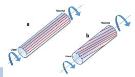
**Figure 3.** Schematic diagram showing the concept of torsion, i.e., the measure of the ability of a material to withstand a twisting load. Torsion is a moment that twists/deforms a member about its longitudinal axis. (a) Stiff catheter (e.g., nylon) with no deformation of longitudinal lines on applying torsion. (b) Non-stiff catheter (e.g., polytetrafluoroethylene) with deformation of longitudinal lines on applying torsion.
